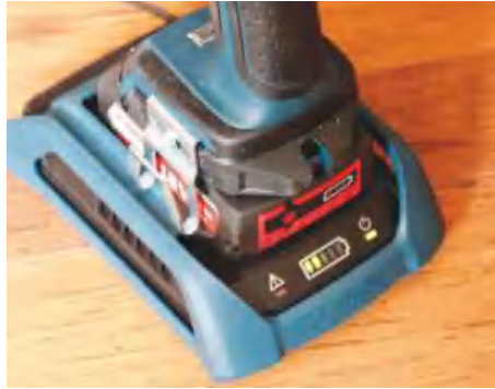
▲ The blue outer cradle allows the battery to slide in and be held securely
